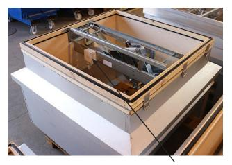
Connect the motor via external cable to the white junction box.
