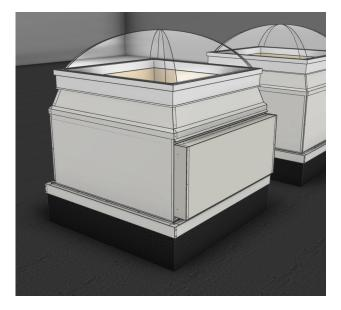
Mount the hatch at the top so that it hooks into the plate and then fold it down until it rests.
